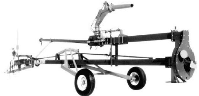
**BOTTOM AGITATION GUNS** - this model is especially effective for use in lagoons with heavy bottom solids, which are common in swine operations. The gun is located near the bottom of the lagoon so that the agitation stream can be directed at the bottom solids to break them up and homogenize them into the lagoon slurry. This allows the lagoon to be managed more effectively and eliminates diminishing lagoon capacity due to bottom sludge build-up.
